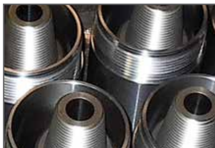
API drill rods and casing subs are typical tooling items
